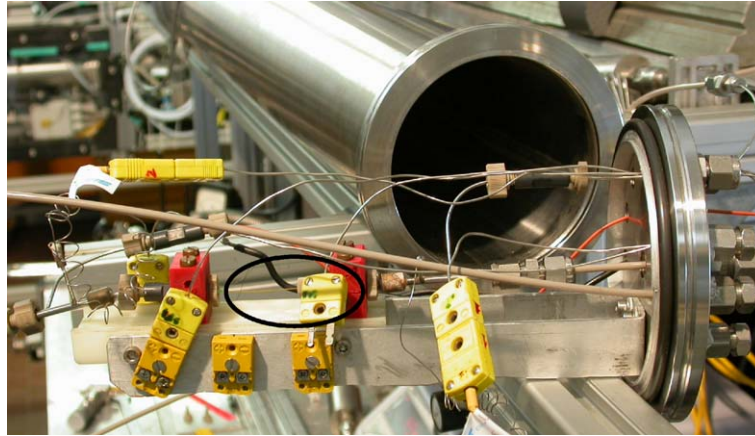
Fig. 4. Close-up of vacuum chamber and flange with mounted test section (circled), thermocouples and pressure ducts.
